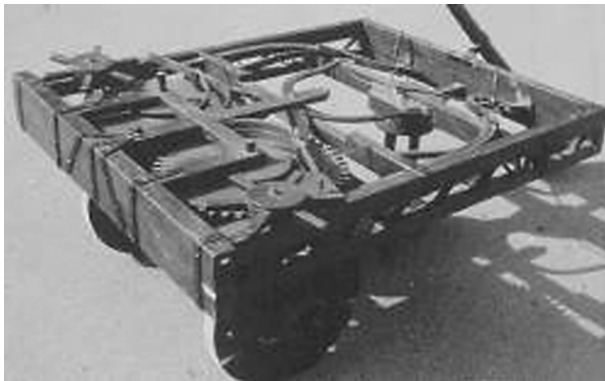
FIG. 3. Mark Rosheim's reconstruction of Leonardo's automated cart (base).
